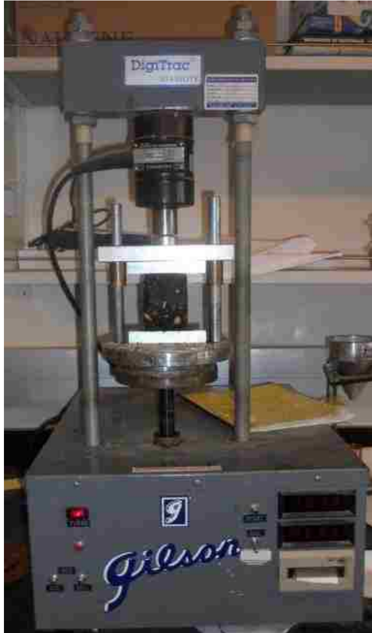
Figure 3.8 IDT testing in progress
