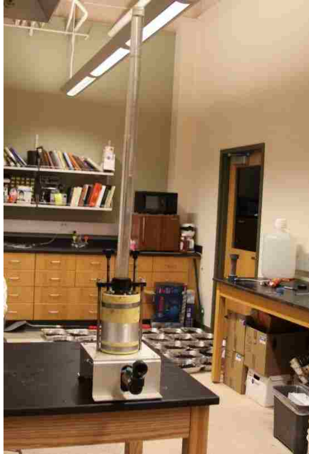
Figure 3.6 Laboratory permeability test
