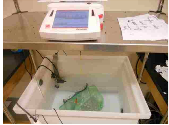
(a) Vacuum sealed sample inside a polybag (b) Weight of sealed sample under water
