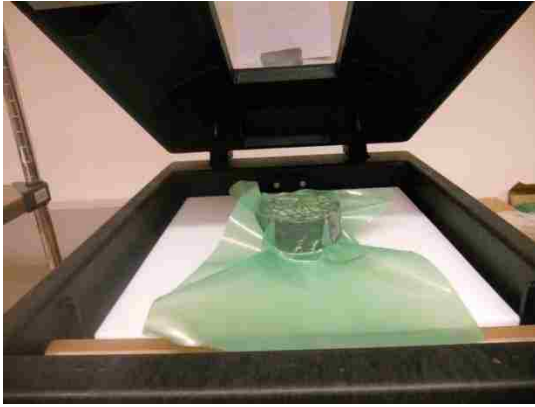
(a) Vacuum sealed sample inside a polybag (b) Weight of sealed sample under water
